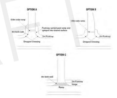
3.38 The junction of a shared private drive onto a Type A, B and C can be formed using a dropped crossing. On higher standard routes, ideally a 4.0 metre radii should be provided. Where access is taken from a Type A Street or a higher standard route, the initial 5.0m section of shared Private Drive should be 5.0m wide.
